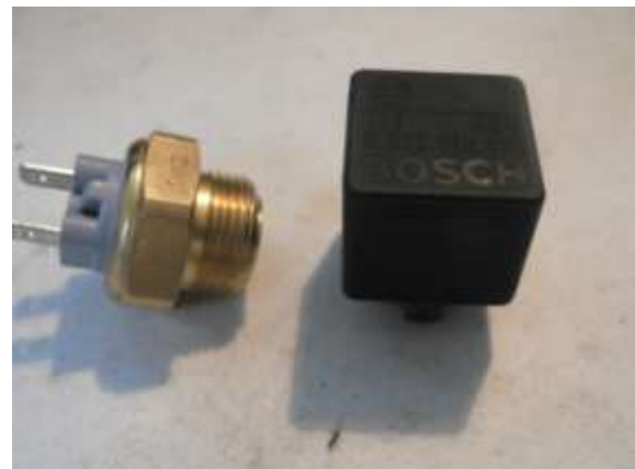
Switch and Relay.
