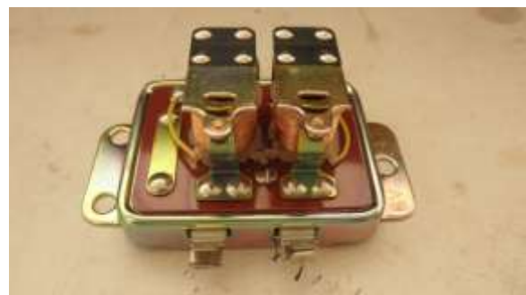
This relay illustrated is a 6 volt double one purchased at a Flea market for R50.00
